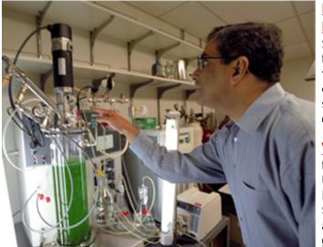
Himadri Pakrasi, Ph.D., professor of biology, explains the photobioreactor in his Rebstock Hall laboratory. Inside the tube, WASHINGTON UNIVERSITY photosynthetic bacteria are making ethanol more efficiently than other forms of biomass because the cvanobacteria are natural
